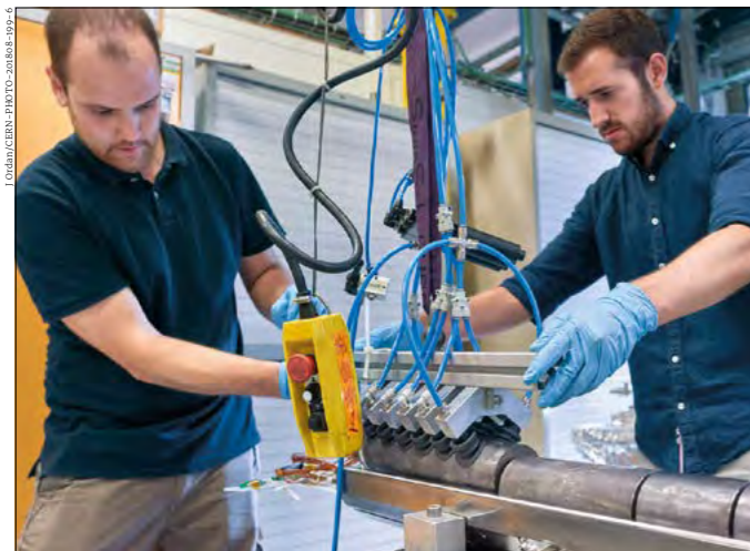
Beam-dump facility Installation of the tantalum-clad pure tungsten block in the Beam Dump Facility prototype target assembly, before testing with proton beam, in 2018.
