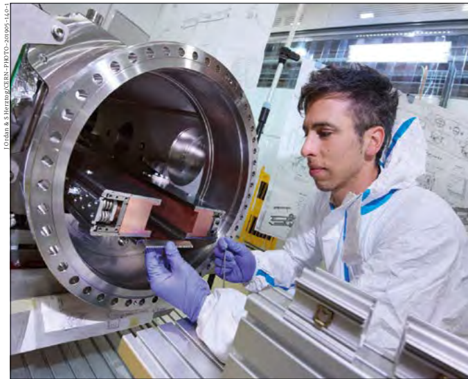
Material integrity test Preparation for irradiation of graphite and copper alloy for the HL-LHC injection dump (TDIS) at the HiRadMat facility in 2018.
